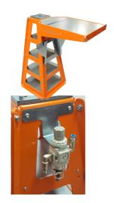
RM-AB: To adjust items accurately on the gripper they can be dropped and re-picked on a alignment wedge.
